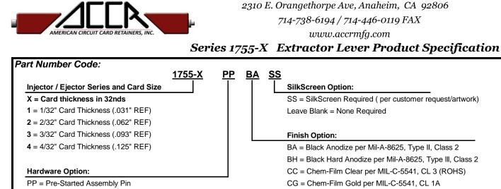
Blank = One Loose Pin (Stainless 3/32" X 1/4") per Lever
